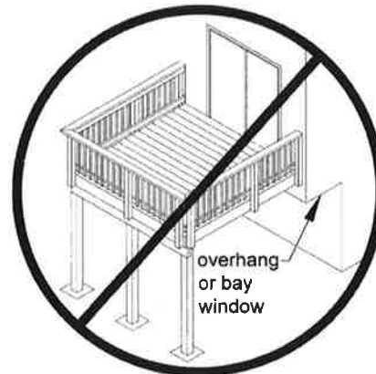
Figure 18. No Attachment to House Overhang with Ledger.
